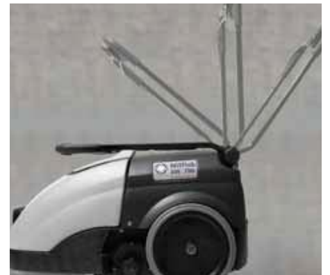
The handle is fully adjustable to suit each individual operator. It folds down completely to simplify storage.
